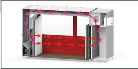
Paint stop filter, secondary filter & carbon filter with clean air filter
